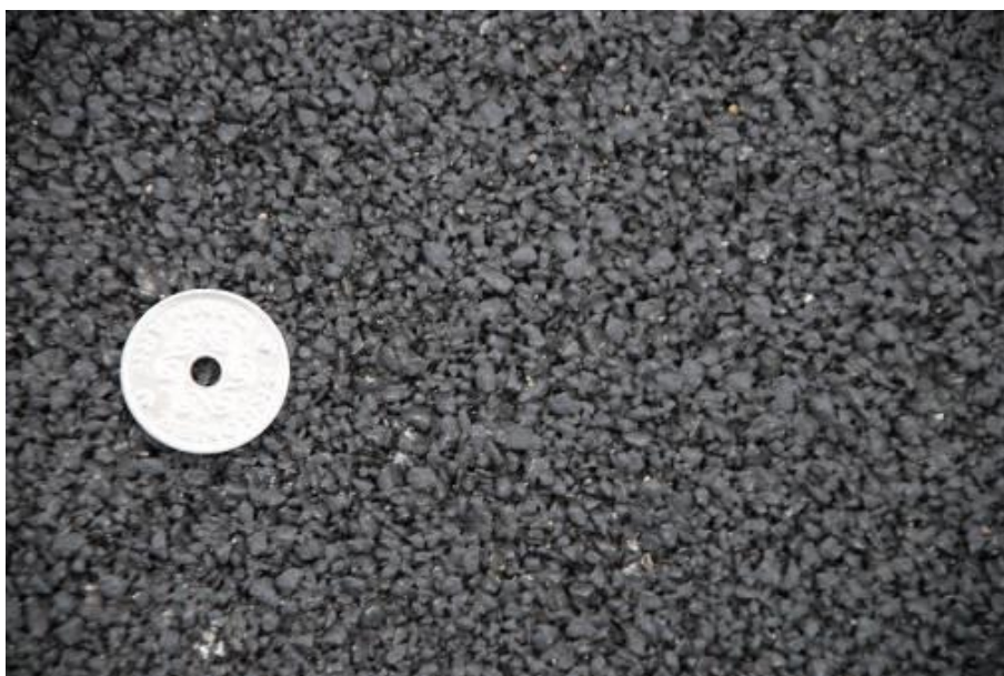
Rys. 11. Nawierzchnia jednowarstwowa (DVS-DRI Super Quiet Traffic International search for pavement providing 10 dB noise reduction, Danish Road Institute Report nr 178, 2009)
